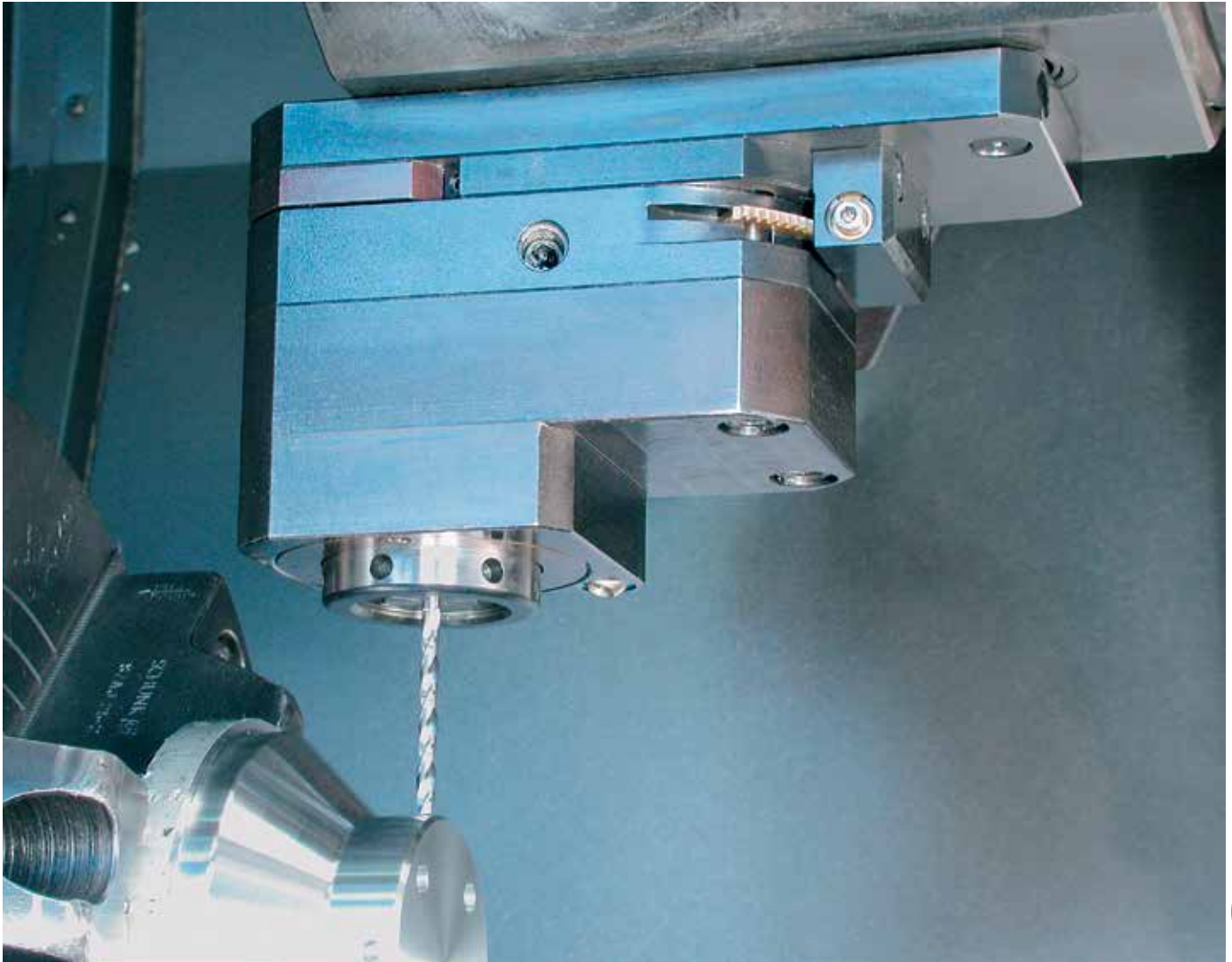
Picture shows a Y-axis live tool with an adjustment range of \pm 50 mm in Y-axis.
