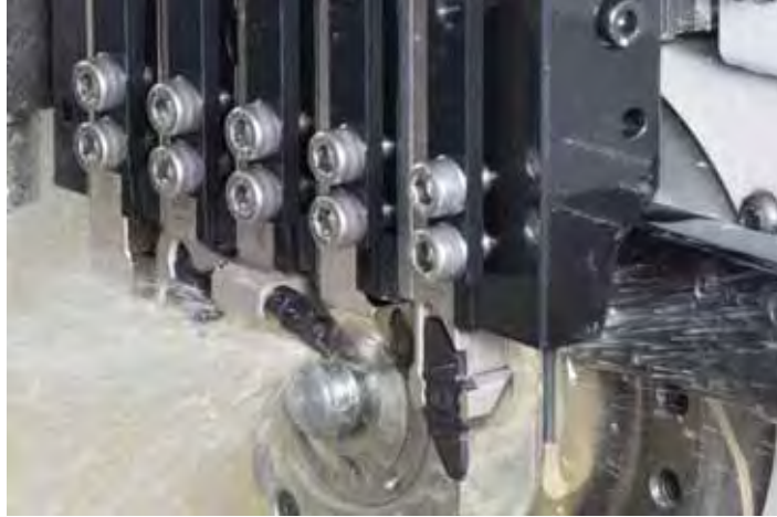
Direct connection without coolant tube
