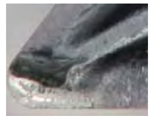
High pressure coolant (7 MPa)
