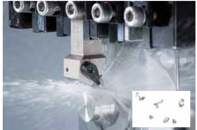
High pressure coolant (7 MPa)
