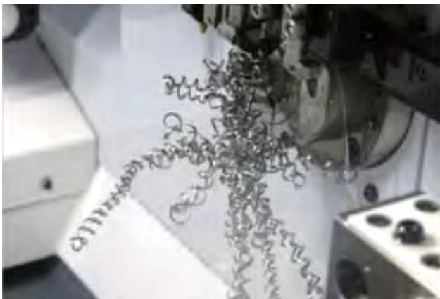
External coolant supply at normal pressure
