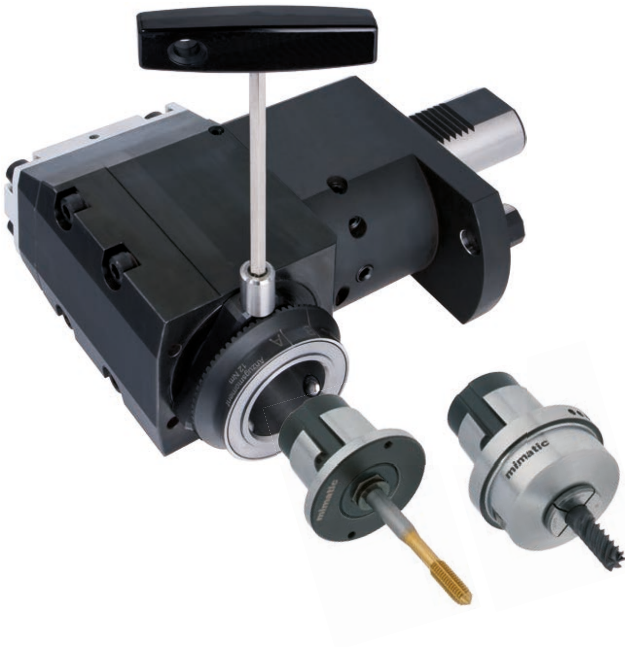
Picture shows a mimatic® 90° angle driven toolholder for Mazak VDI 40 with modular quick change system „mi“. The mimatic® mi interface is a very innovative modular quick change system to reduce machine downtimes because all units can be preset outside the machine.
